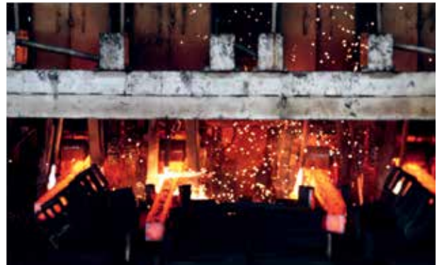
Continuous Casting Machine
